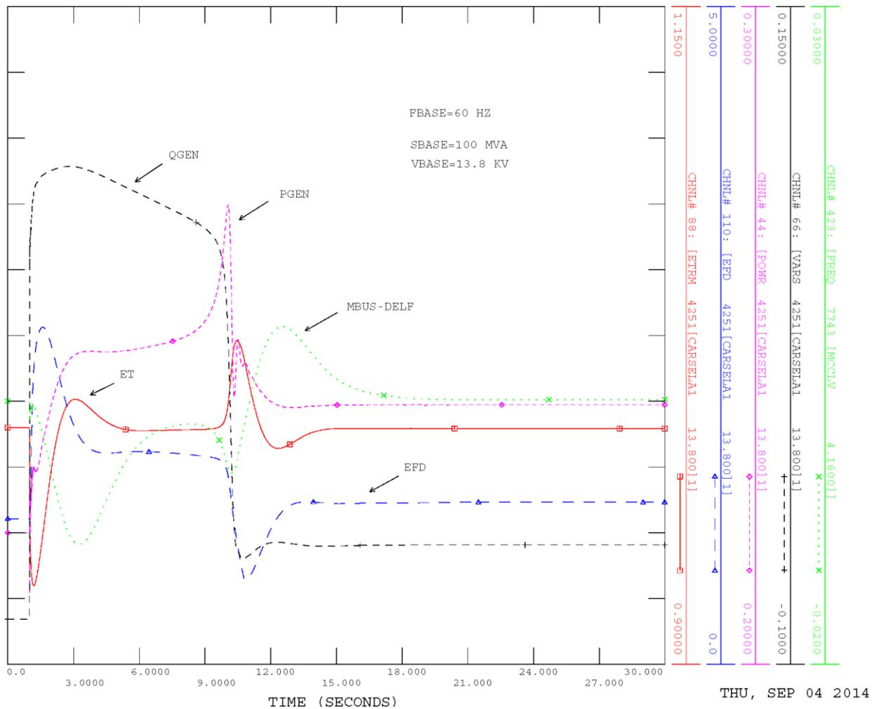
**Figure 5. Blackstart Unit Terminal Voltage, Field Voltage, Reactive Power, Active Power and Frequency Deviation**
