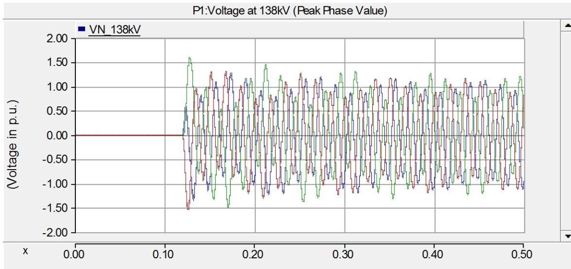
**Figure 3. Example of a Temporary Overvoltage in Per Unit of Nominal Peak Phase Voltage Rating**
