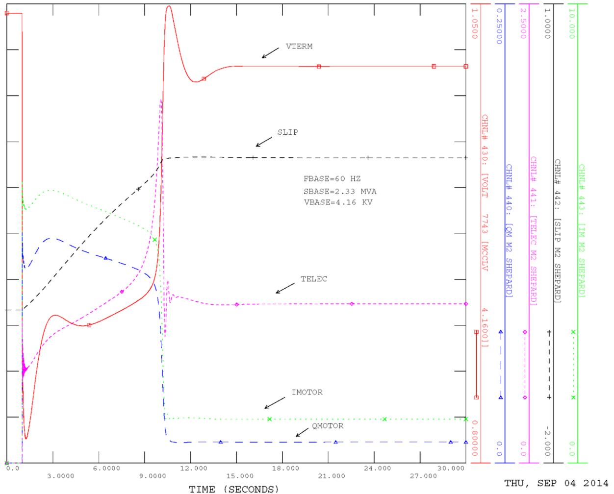
**Figure 4. Motor Terminal Voltage, Reactive Power, Electric Torque, Slip and Current**
