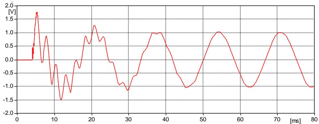
**Figure 2. Example of a Switching Surge from an Electromagnetic Transient Program Simulation of the Energizing of a Typical Overhead Line. The voltage is in per unit of the nominal peak phase voltage rating.**
