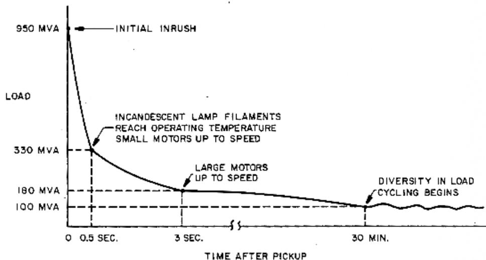
**Figure 1. Load Variation Following Cold Load Pickup**
